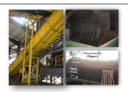
Separating the fruit from the bunch - truck loaded with baked palm to Tipper to pour out on to the conveyor belt to the Threshing Machine to separate the fruit from the fruit bunch then the fruit is transported by conveyor to the fruit oil extractor while the empty fruit bunch is transported by conveyor to the fruit bunch oil extractor.
